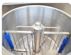
Removable tool with integrated bowl scrapers
